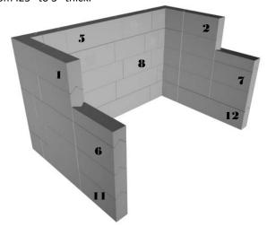
This cave demonstrates the dimensions and variations of bricks available for a lead cave. The construction of an interlocking enclosure requires careful calculation to ensure stability.
